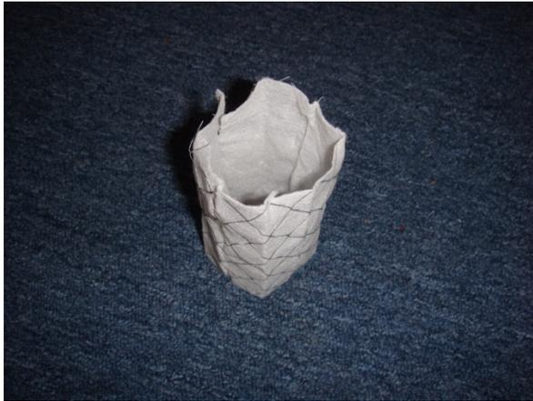
Figure 8 | Single walled pleated air filter in vertical orientation
